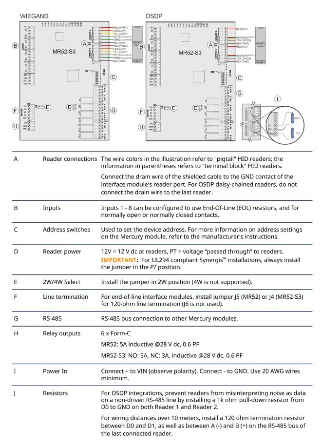
To find out whether you need to add a 1K ohm pull-down resistor between D0 and GND, see KBA-78953.
